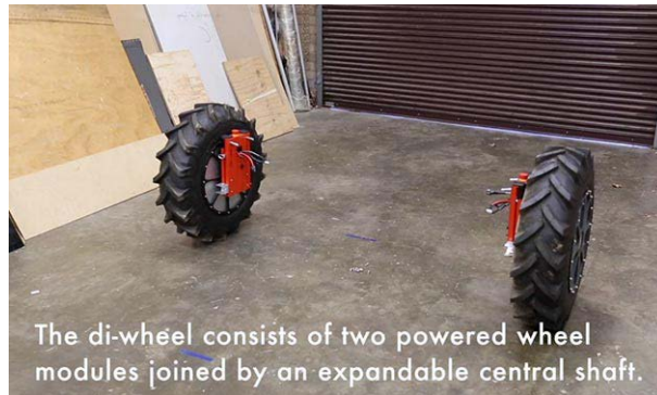
Figure 4. First iteration of the Digital Farmhand: the di-wheel.
